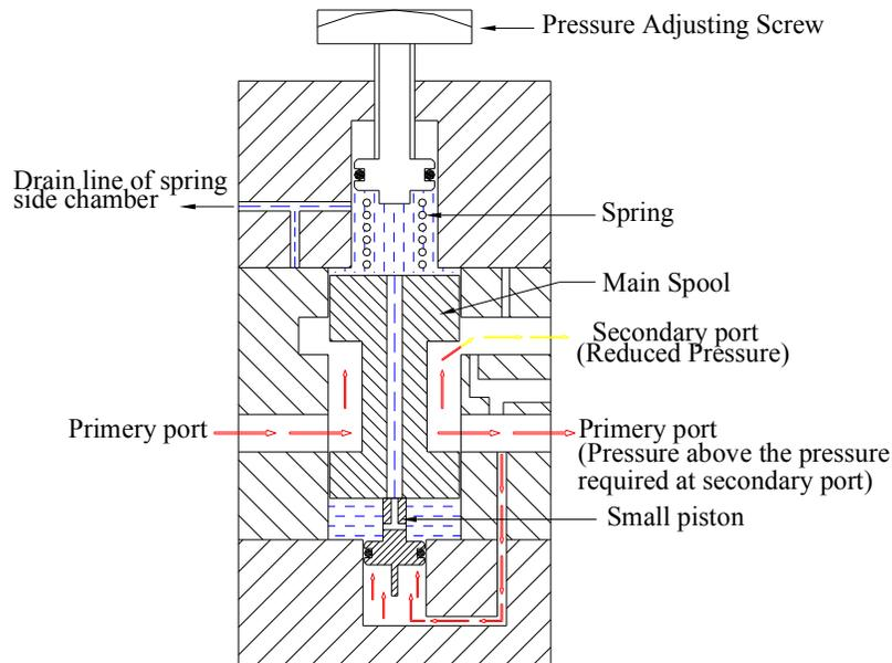
As primary side pressure rises above spring setting secondary part open slightly
