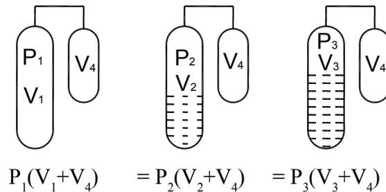
Accumaltor capacity = V<sub>f</sub> = V<sub>2</sub> - V<sub>3</sub>
