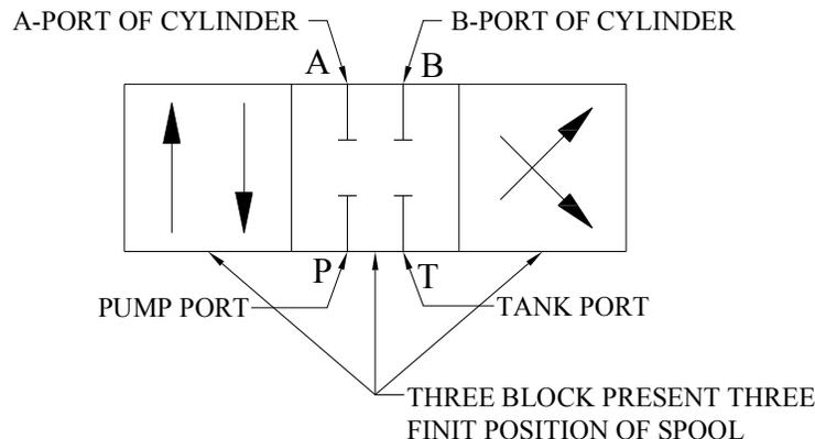
This diagram indicates at central position all ports will be blocked as we studied in circuit diagram. (30.2) On its one (left) extreme end pump will be connected to port-A and tank is connected to port-B. On its other (right) extreme end pump will be connected to port-B and tank is connected to port-A.
