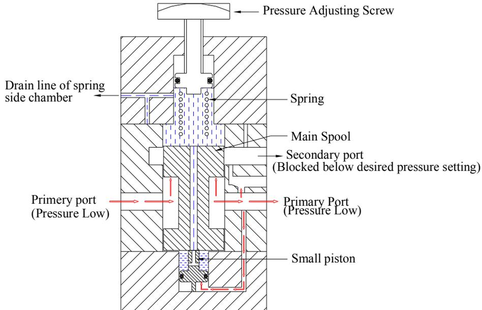
Secondary side pressure line blocked as primary side pressure is below the required
