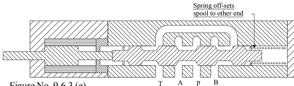
**4. Two Position Actuated to Center:** - In this configuration also spring offset spool to actuator extreme end. But when spool actuated it comes center position. It cannot pass on to spring extreme end.
