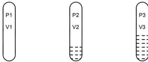
Recharged condition      Minimum fluid level in accumulator      Maximum fluid level in accumulator
