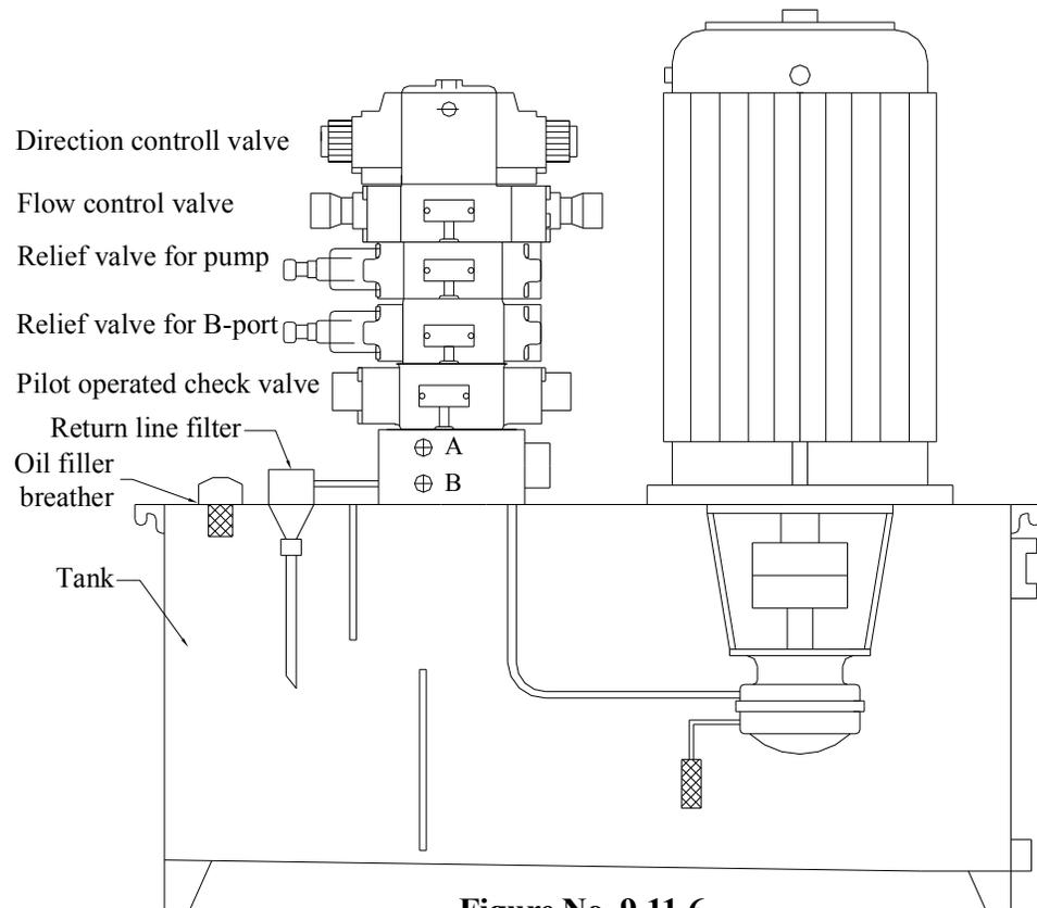
In following example we have added many modular valves such as, flow control valve, pilot operated check valve, pressure relief valve for both A & B port. The valve used in said power pack unit add following feature in power pack.
