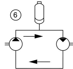
**7) Heavy load suspension:-** Suspension of heavy vehicle are connected to accumulator to absorb heavy shock and maintain pressure in suspension
