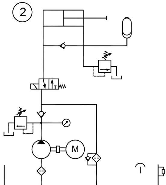
**3) Energy and safety:-** An accumulator which is kept always in fully charged condition, gives instant power for safety operation, such as breaking, closing or opening of door etc. (Pump take few seconds for developing rated pressure, while accumulator keeps it in ready stock for instant supply.)
