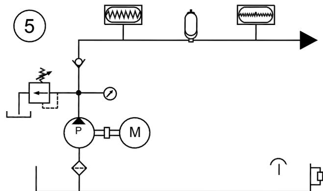
Accumulator dampens the pulse generatd by pump.
