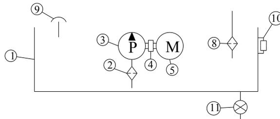
A layout should be made to decide how to fit motor, pump assembly, manifold block, return line filter, air-breather, pressure gauge etc. They should be decided, before fixing of motor-pump assembly. Once layout finalized then motor, pump assembly, and other accessories should be fixed accordingly.
