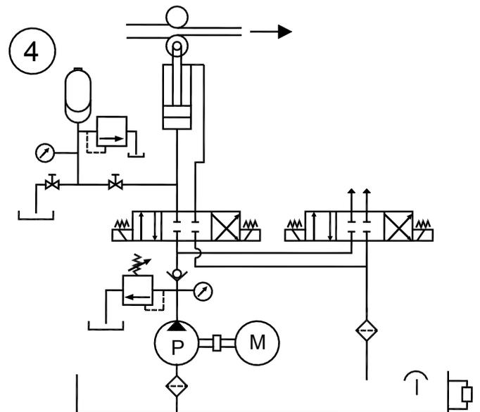
Accumulator supply costant pressure on rolls of rolling machine.
