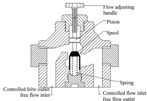
Sub-plate type construction of
