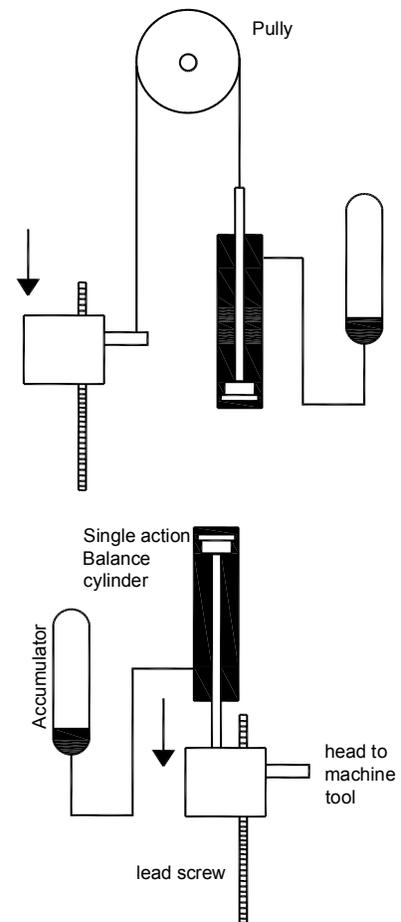
**9.10.5. Calculation for determining Accumulator capacity:-**
