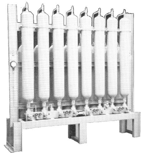
Transfer barriers accumulators are those in which compressed gas section of accumulator is not locked, but connected to pressurised gas bottles or othersource of pressurised fluid.
