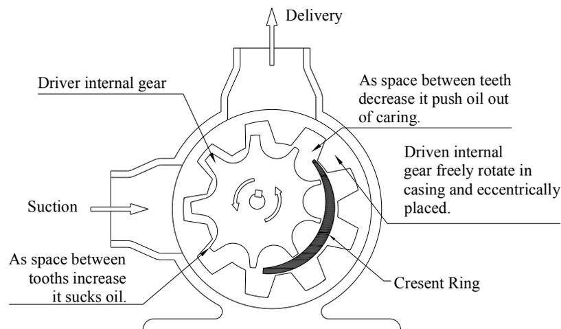
**Internal Gear Pump**
