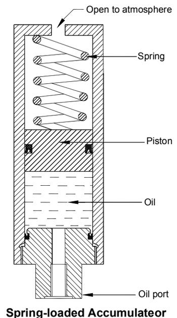
$$\text{Oil pressure in accumulator} = \frac{\text{Spring force}}{\text{Piston force}}$$
