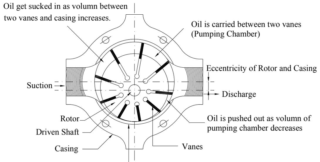
The inside surface of casing is harden-ground and given a special curvature for best performance. (Generally a harden and ground ring called Cam-ring is fitted inside for convenience in maintenace and replacement of worn out ports)
