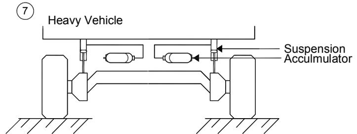
**8) Shock Absorption:-** When a machine part moved by hydraulic, stops suddenly. it generate a shock wave (a peak pressure) in system. An accumulator used in system absorbs such pressure surges. For example: impact test benches, over-head crane etc.
