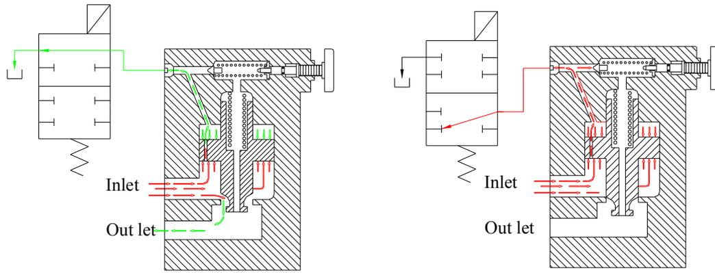
(1) Vent port connected to tank through solenoid valve. Because of which pilot operated relief valve unloading full discharge of pump to tank, and there is no pressure in hydraulic system.
