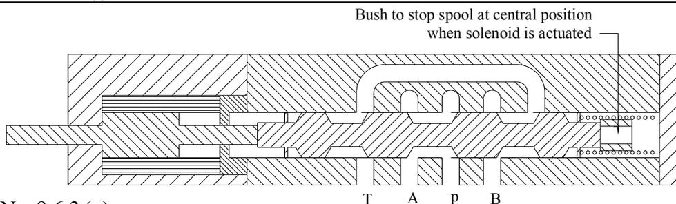
**5. Two Position Detente:** - Similar to the three position spring centered valve this valve also have two actuator but without spring. And it has arrangement to keep the spool to its extreme end even when actuator released. Hence when actuator is shifts the spool it remains in same position, do not return to neutral position even when actuation released. And will pass on to other extreme position when other actuator actuated.
