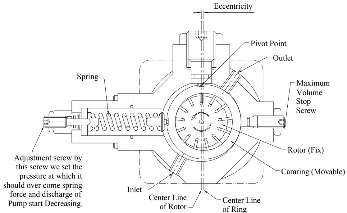
Variable Discharge Vane Pump
