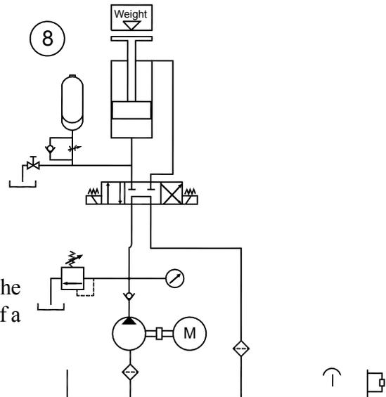
Accumulator connected to cylinder, absorbs the shock generated by impact or sudden stopping of a moving object.
